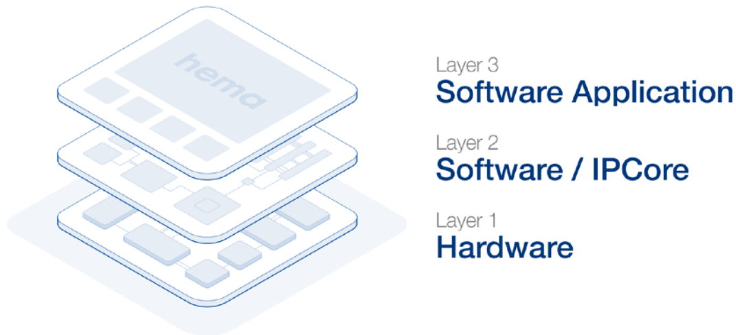
Image 01: SoM based solutions are developed around a three layer model, consisting of hardware, software / IP-Cores and software applications.
